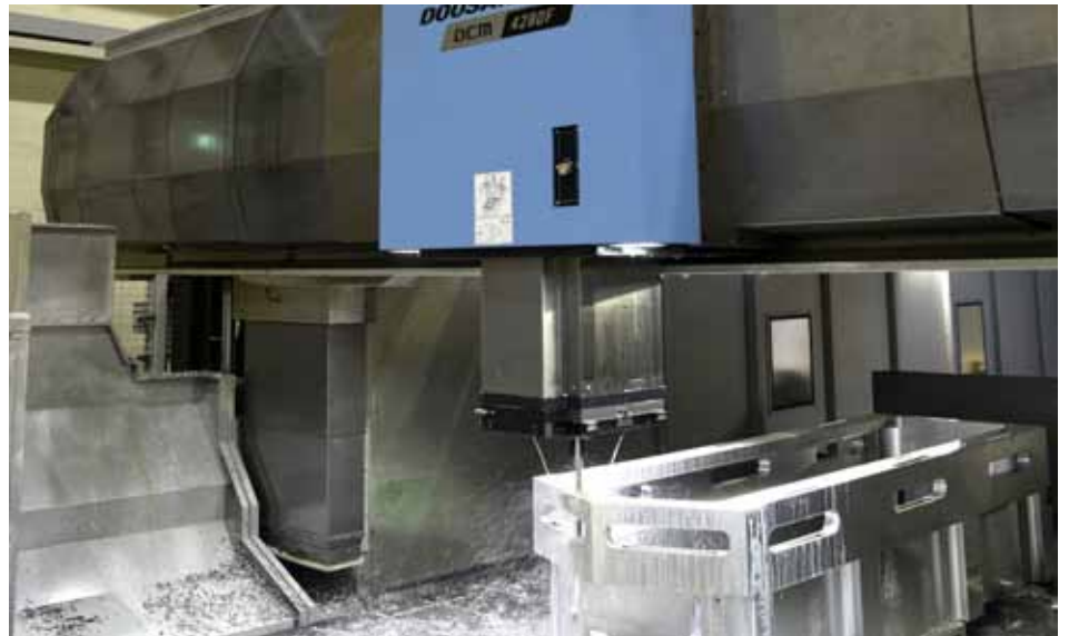
⊕ Dream Mecatec uses the DCM series in its chamber-machining of semiconductor manufacturing equipment requiring heavy cutting and a high degree of accuracy.
